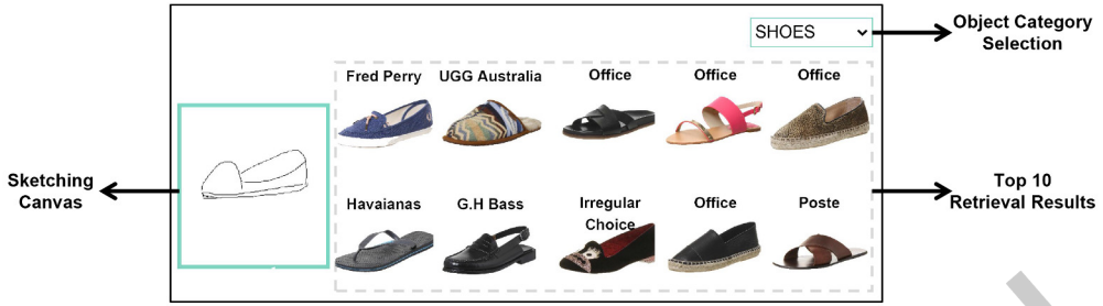
Fig. 2. A snapshot of the user interface of Sketch Me That Shoe [51]. It has an object category selection button at the top, a sketching canvas on the right, and an image display panel at the bottom left. Users are allowed to draw a sketch in their minds to search for an image of shoe. The top 10 retrieved images are shown.
