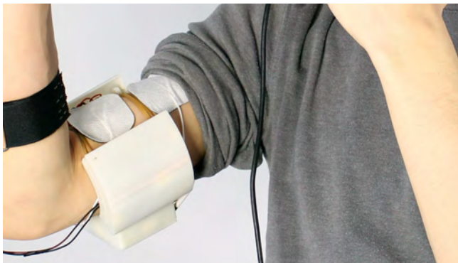
Figure 3: Detail of the electrical muscle stimulation component. Here, it stimulates the user’s biceps brachii muscles causing an involuntary contraction that resembles force feedback.
