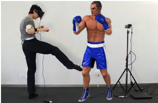
Figure 11: Combining impacto units on arms and legs allows us to support a simple Thai Boxing experience.
