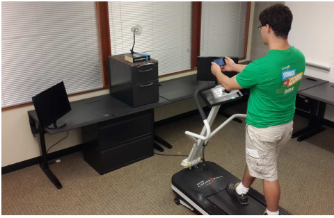
Figure 7. To support the different conditions, the experimental setup included a treadmill for walking, a lamp for consistent lighting, and a monitor on either side for distractions.
