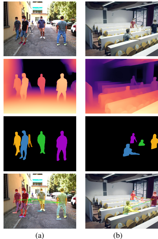
Fig. 1. Monitoring social distancing from images. Images concerning outdoor (a) and indoor (b) environments. From top to bottom: reference RGB image, estimated depth, segmented people, and estimated inter-personal distances, with the color (red, orange, green) of the segment denoting the class of risk (dangerous, risky, safe), as explained in Section IV-D. In contrast to most other methods, our framework reliably estimates the inter-personal distance without constraints about the sensed environment even when dealing with multiple and not visible ground planes (b).
