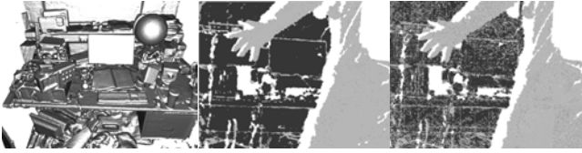
Figure 7: Example of point-plane outliers as person steps into partially reconstructed scene (left). Outliers from compatibility checks (Equation 17) using a surface measurement with (center) and without (right) bilateral filtering applied to the raw depth map. \Omega(\mathbf{u}) = \text{null} are light grey with unpredicted/unmeasured points shown in white.
