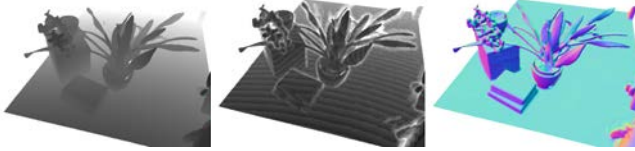
Figure 6: Demonstration of the space skipping ray casting. (Left) pixel iteration count are shown where for each pixel the ray is traversed in steps of at most one voxel (white equals 480 increments and black 60). (middle) ray marching steps are drastically reduced by skipping empty space according to the minimum truncation \mu (white equals 70 iterations and black 10 \approx 6\times speedup). Marching steps can be seen to increase around the surface interface where the signed distance function has not been truncated. (Right) Normal map at resulting surface intersection.
