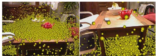
Figure 14: Thousands of particles interact live with surfaces as they are reconstructed. Notice how fine-grained occlusions are handled between the real and virtual. Simulation works on the TSDF volumetric representation, and runs on the GPU alongside tracking and mapping, all in real-time.
