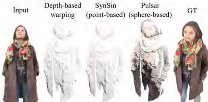
Fig. 2. Comparison of 3D point cloud transformations. From a single RGB-D input, we obtain the warped image using: a depth-based warping transformation [34,40], the neural point-based renderer SynSin [64] and the neural sphere-based Pulsar renderer [33]. The novel image warped by Pulsar is significantly denser.
