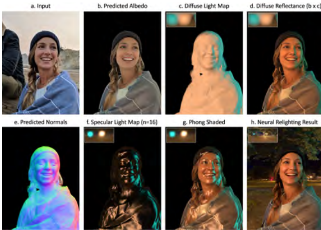
Fig. 6. For an input portrait (a), we first infer surface normals (e) and albedo (b). Given a target HDR lighting environment and the normals, we compute the diffuse and specular light maps (c, f). Multiplying (b) by (c) yields approximate diffuse reflectance, without self-shadowing, while (f) suggests the locations of specular reflections for the new scene, as shown in the Phong-shaded subject in (g). Our neural relighting module learns to recover self-shadowing and specularities, as shown in result (h), beyond what can be rendered using the simple shading model of (g or d).
