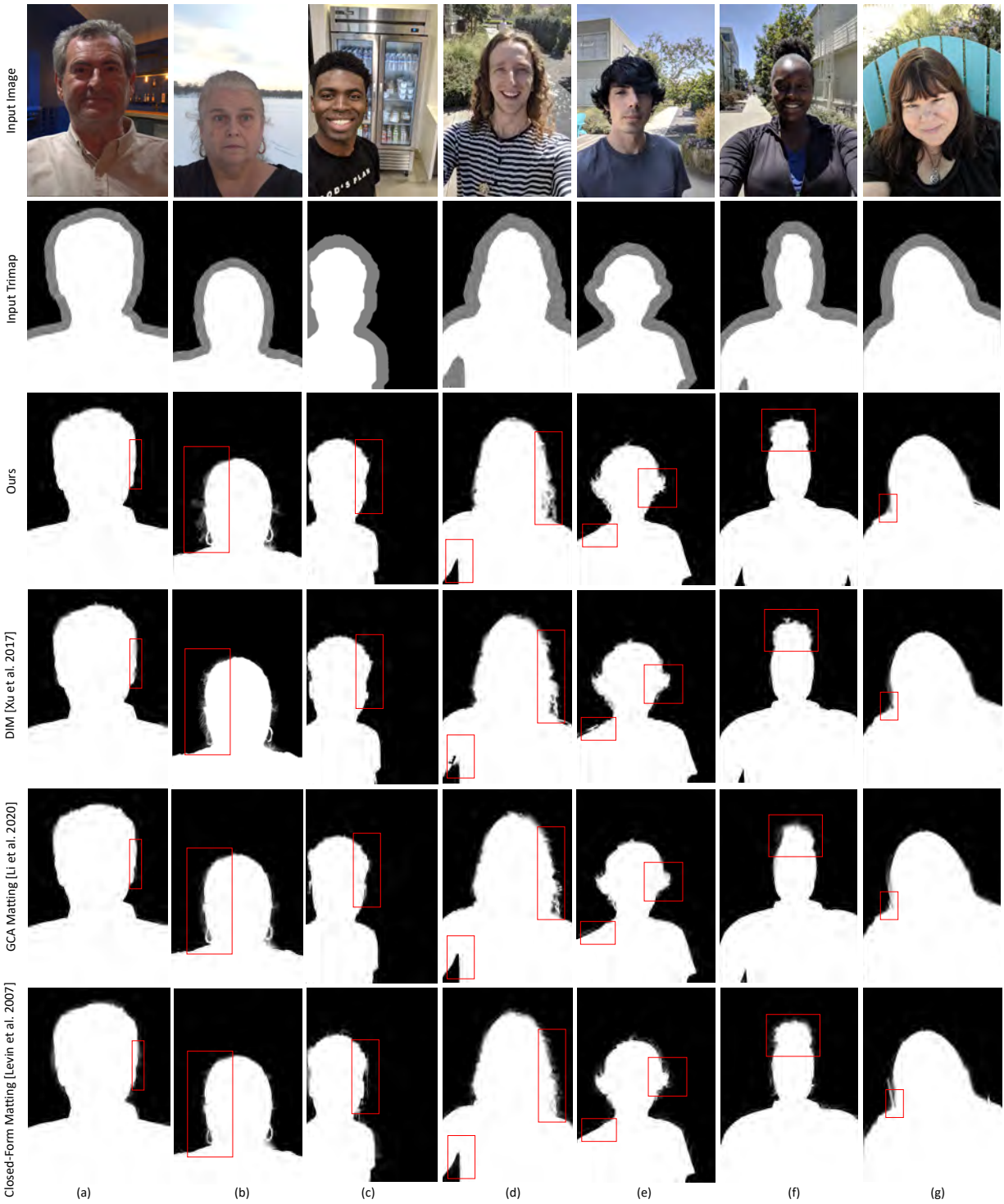
Fig. 13. (a,b): Estimated alpha mattes for evaluation images made by compositing light stage images. (c-g): Estimated alpha mattes for in-the-wild images. Note how the proposed matting module better generalizes on in-the-wild-images when compared with state-of-art pre-trained models using Adobe-1k and alphamattng.com datasets.
