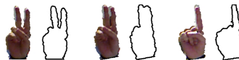
Figure 1: Some challenging cases for hand gesture recognition, using depth cameras: the first and the second hands have the same gesture while the third hand confuses the recognition.
