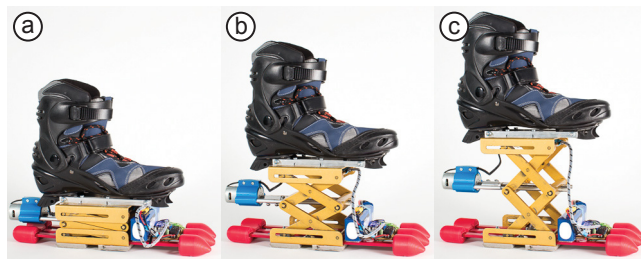
Figure 3: A Level-Up actuating its scissor mechanism
