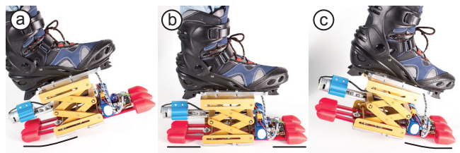
Figure 6: Fiberglass gives the artificial foot its flexibility
