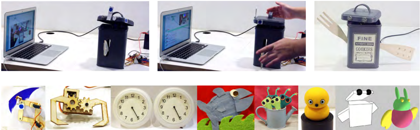
Figure 1. Mirror Puppeteering is a system for creating gestures for a robot by moving its limbs in front of a webcam. First, a robot tagged with markers self-calibrates in front of a webcam, building up a map between motor angles and camera-space marker locations ( top left ). The user then creates animations by puppeteering the robot's limbs in realtime ( top middle ). Animations are played back by the stand-alone robot ( top right ), or can be transferred to control animated characters. We demonstrate our system on a variety of homemade robots, the commercial toy My Keepon, and two virtual characters ( bottom row ).
