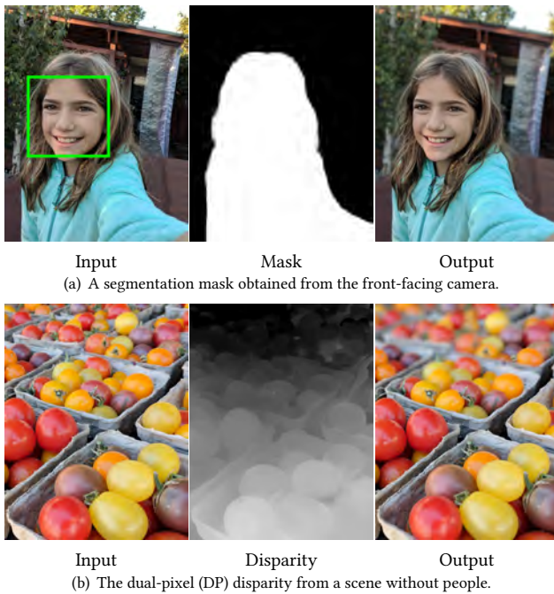
Fig. 2. Our system gracefully falls back to one of the two inputs depending on availability. On the front-facing camera (which lacks dual-pixels), the image is almost always of a person in front of a distant background, so using the segmentation alone is sufficient (a). For close-up shots of objects, disparity data from dual-pixels alone is often sufficient to produce a high-quality output (b).
