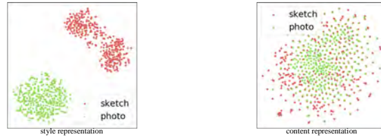
Fig. 9: The style representations of sketches and photos are well separated, while the content representations of sketches and photos are tangled together. We visualize learned content and style representations of sketches and photos with T-SNE [25]. The results show that sketches and photos share the content space and it is appropriate to train on photos and transfer knowledge to sketches.
