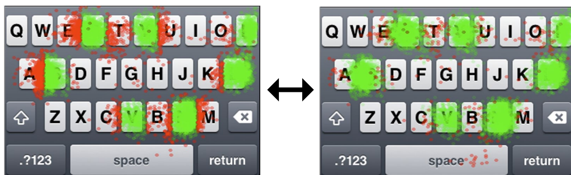
Figure 2. The benefits of the WalkType keyboard. Green dots represent correct keypresses. Red dots represent errors. The left keyboard naively classifies based on key boundaries, while the right keyboard uses WalkType to achieve 45.2% fewer errors on the same data. (Neither keyboard has any natural language processing features enabled in order to isolate the effects of WalkType on the keypress locations alone.) Figure adapted from prior work [10] with permission from the authors.
