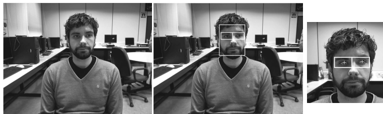
Fig. 2. The detection scheme: the face is first detected, and then the eye regions are roughly estimated. The iris center detection algorithm is applied to each eye image.
