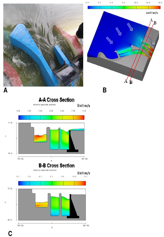
**Figure 7.** Flow distribution at the approach channel in PMF. A. Hydraulic model test; B. Numerical simulation; C. Cross section view.
