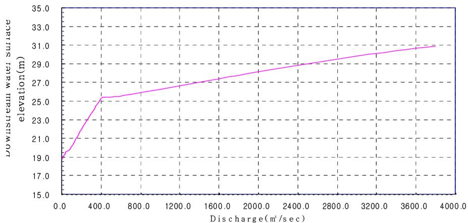
**Figure 5.** Stage-discharge relation curve of the downstream river.
