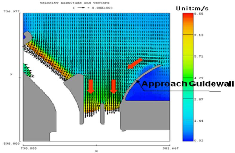
**Figure 9.** Two dimensional flow velocity distribution at the approach channel based on revised plan design (Flow velocity distribution at depth EL. 68.12 m).
