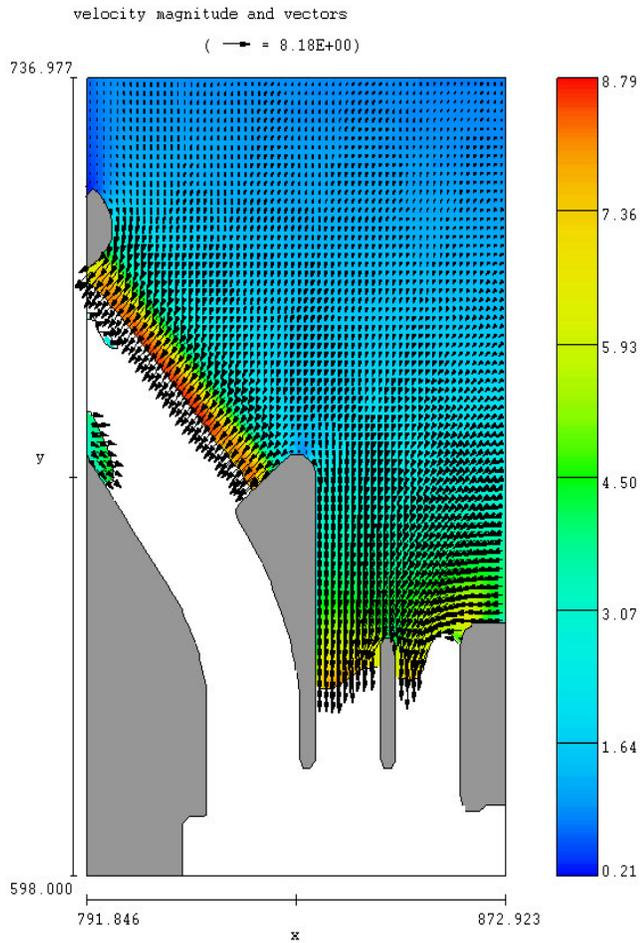
**Figure 6.** Two dimensional flow velocity distribution at the approach channel (Flow velocity distribution at depth EL. 68.12 m).
