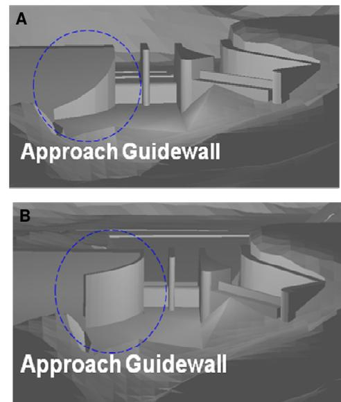
**Figure 8.** Revised approach channel section. A. Initial plan design; B. Revised plan design.
