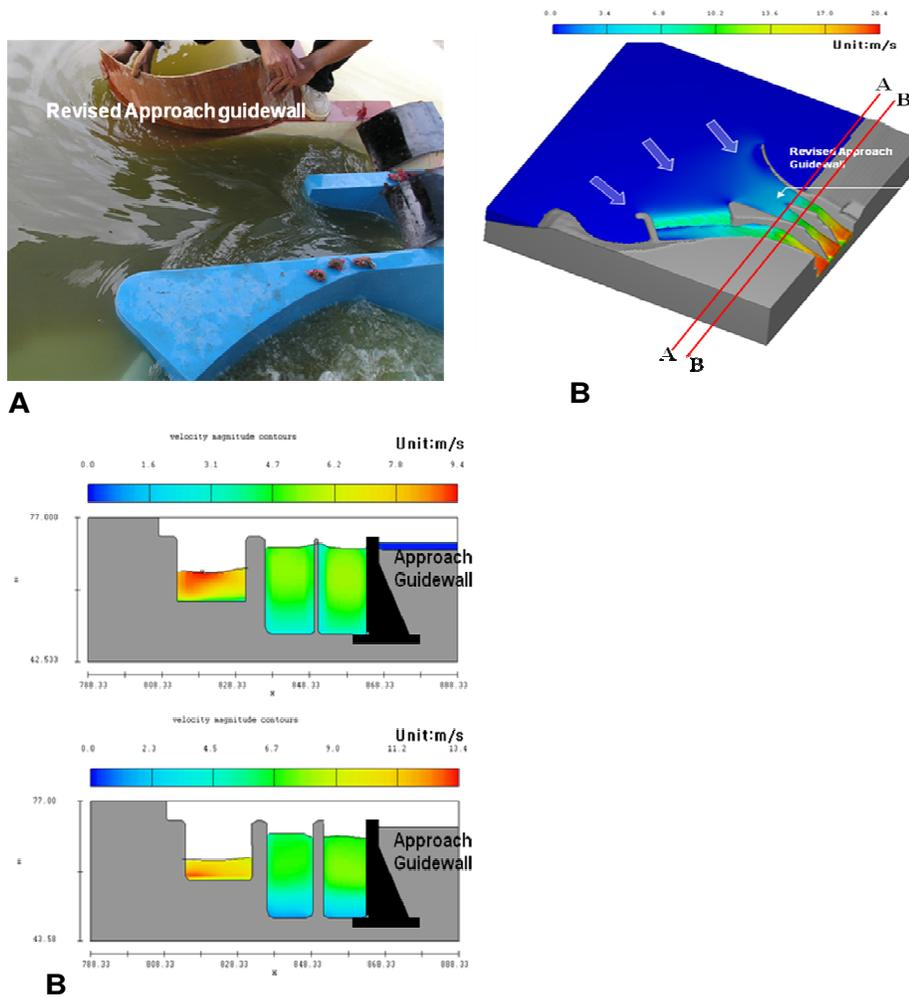
**Figure 10.** Flow distribution at the approach channel in PMF based on revised plan design. A. Hydraulic model test; B. Numerical simulation; C. Section view.
