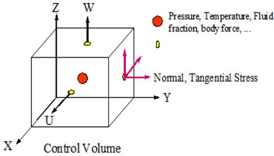
Figure 1. Grid system for a FLOW-3D.
