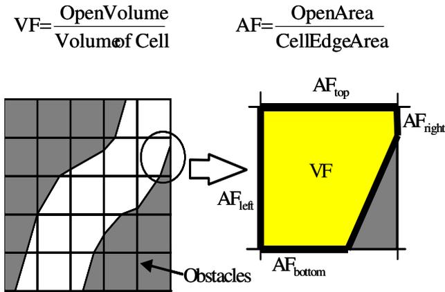
Figure 2. Conceptual diagram of a FAVOR method.
