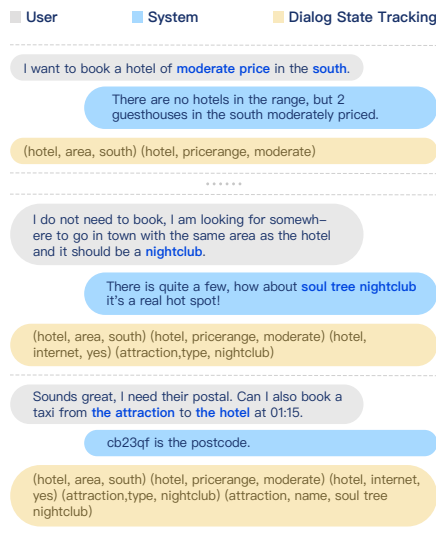
Figure 1: An example of dialogue state tracking process for booking a hotel, looking for an attraction and booking a taxi between them. Each turn contains a user utterance (grey) and a system utterance (blue). The dialogue state tracker (yellow) tracks all the ( domain, slot, value ) until the current turn. Blue color texts indicate mentions of slot values appeared at that turn. Best viewed in color.
