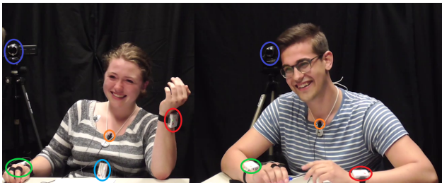
Figure 1: An example of participants interacting during one of the sessions of the experiment, all visible sensors are encircled. Each color represents a different kind of sensor (indigo = over-the-shoulder cameras, turquoise = EXG+ units, red = regular IM units, green = GSR+ units and orange = lavalier microphones)
