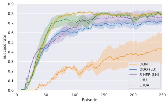
Figure 3: Comparisons between LHUA and its ablations: DQN (no hindsight manager, no user modeling, and no adaptive coordinator), DDQ (no hindsight manager, and no adaptive coordinator), S-HER (no user modeling, and no adaptive coordinator), and LHU (no adaptive coordinator). A complete LHUA includes all the components, including DQN (for naive dialog policy learning), hindsight manager, user modeling, and adaptive coordinator.
