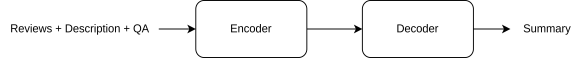
Figure 4: Framework of the baseline model that takes reviews , description , and QA as the input. A simple concatenation (+) of the input sources is used to generate a summary. During inference, the model generates a summary whereas during training the model uses pseudo-summary obtained through SDC process for learning.
