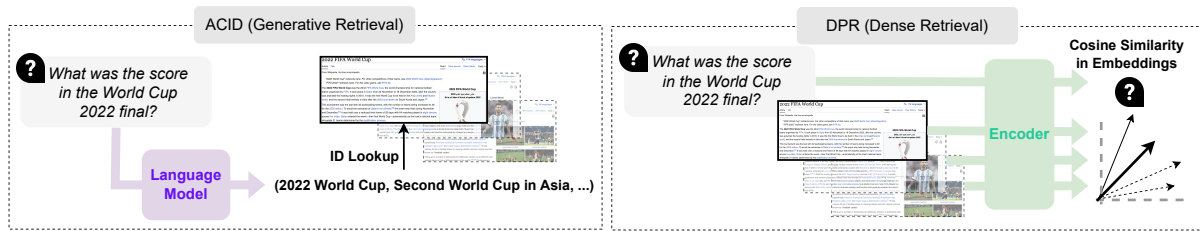
Figure 1: Generative retrieval vs. dense retrieval. In dense retrieval (right), both the query and the documents are encoded into dense vectors (i.e., embeddings). Nearest-neighbor search is then applied to find the most relevant documents. Generative retrieval (left) trains a language model to generate the relevant document ID conditional on the query. The ID is tied to a unique document, allowing for direct lookup. We propose summarization-based document IDs like ACID, which uses GPT-3.5 to create a sequence of abstractive keyphrases to serve as the document ID.
