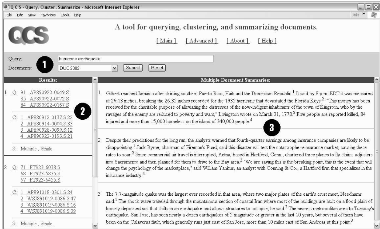
Figure 1: The interface to the QCS system includes 1) an input section for the query and choice of document set, 2) a navigation section with links to clustered documents (Q: top documents retrieved for the query and their scores, C: documents from which summary sentences were drawn and the sentence indices, S: links to multiple or single document summaries), and 3) an output viewing section, which here contains the default output of multiple document summaries for the topic clusters.
