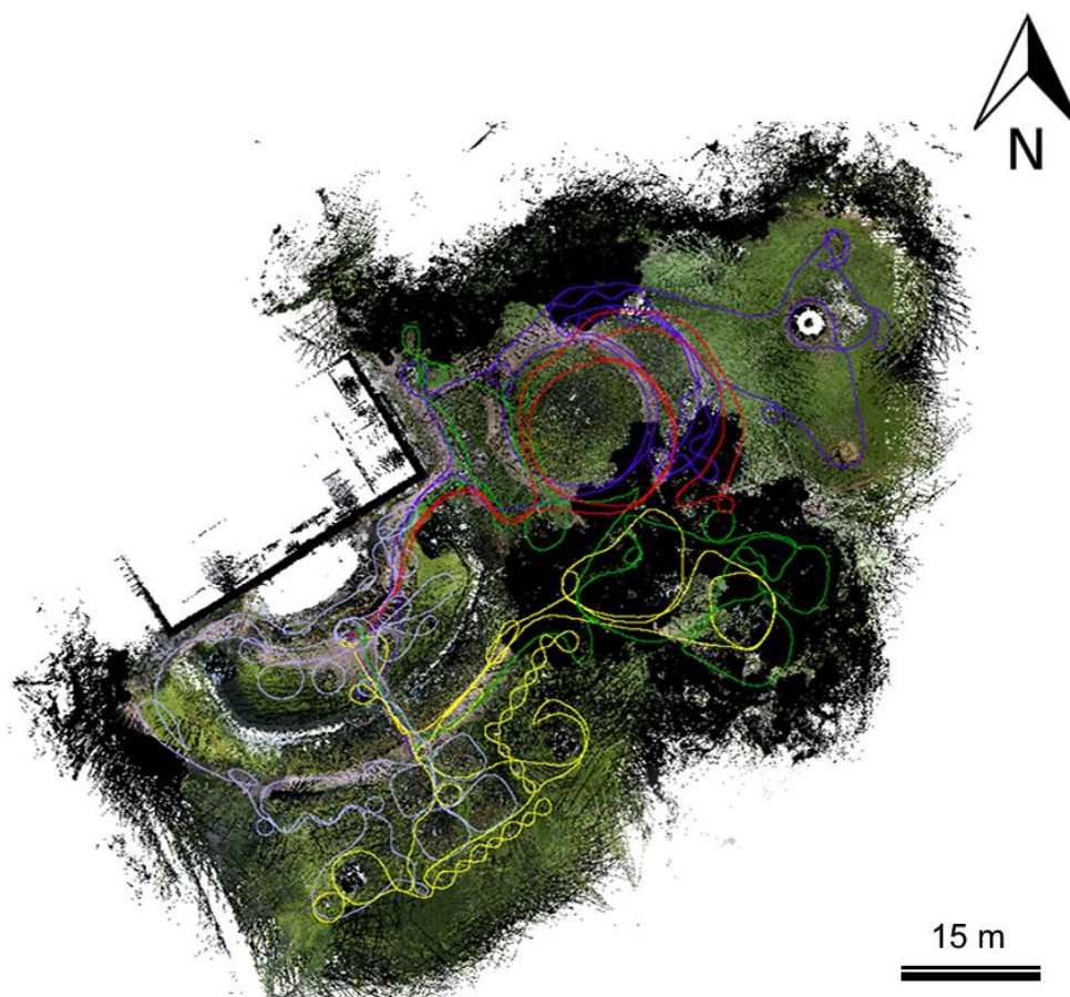
Figure 4. CoSEAM ZER Rev. RT point cloud with independent measurement trajectories which are colored individually as blue, red, yellow, green, and purple. The point cloud is colored with the data of the integrated camera system, and the black points are laser scanning points that do not have any color value from camera data.
