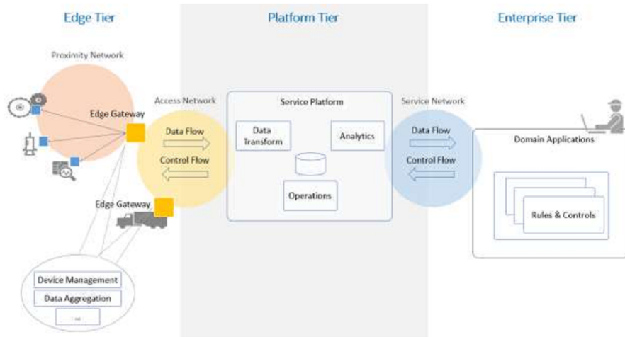
Figure 8-4: IIC three tier IIS architecture
