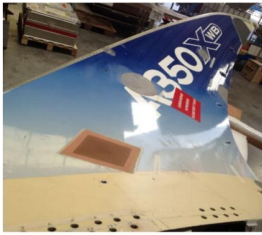
Example of bonded repair
