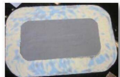
Example of Cosmetic Permanent repair – restoration of ECF
