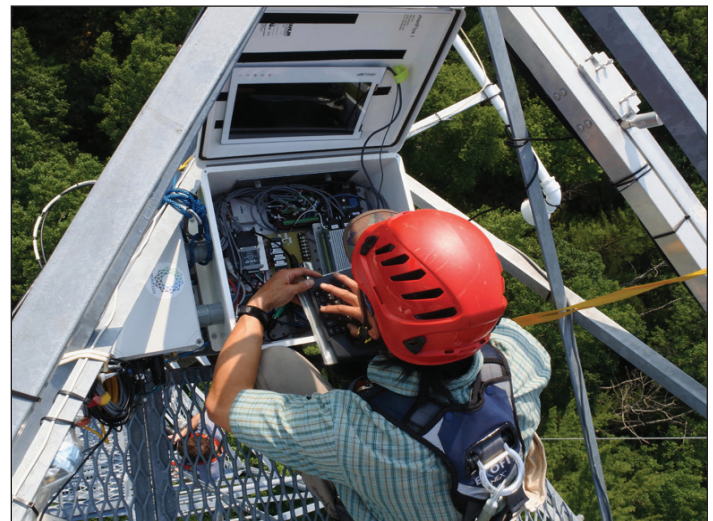
Ameriflux Tech Team. Stephen Chan checking the Ameriflux portable eddy covariance system (PECS), comparing data to that of the Ameriflux US-UMB site's eddy covariance system. Photo credit: Chris Vogel.
