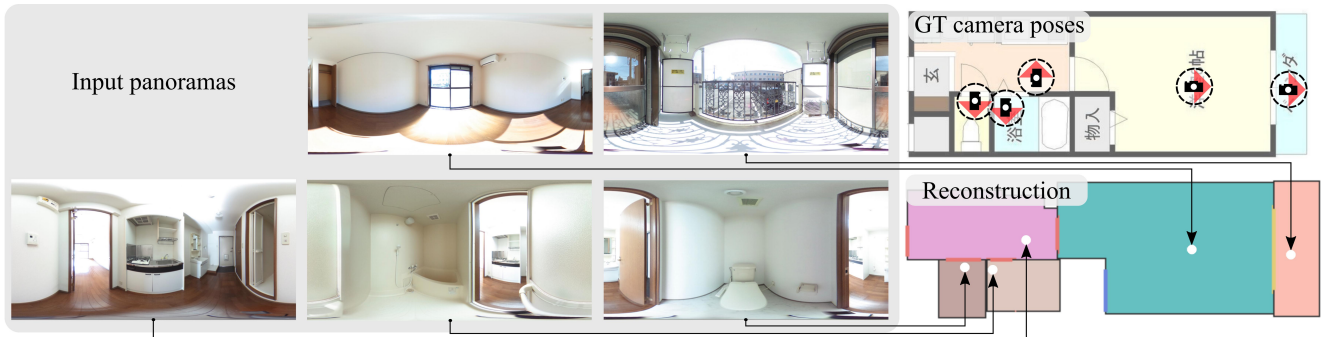
Figure 1. The paper introduces an extreme Structure from Motion problem for indoor panoramas that have little to no visual overlaps. Our approach learns to evaluate the realism of room/door/window arrangements in the top-down semantic space and solve for the camera poses.
