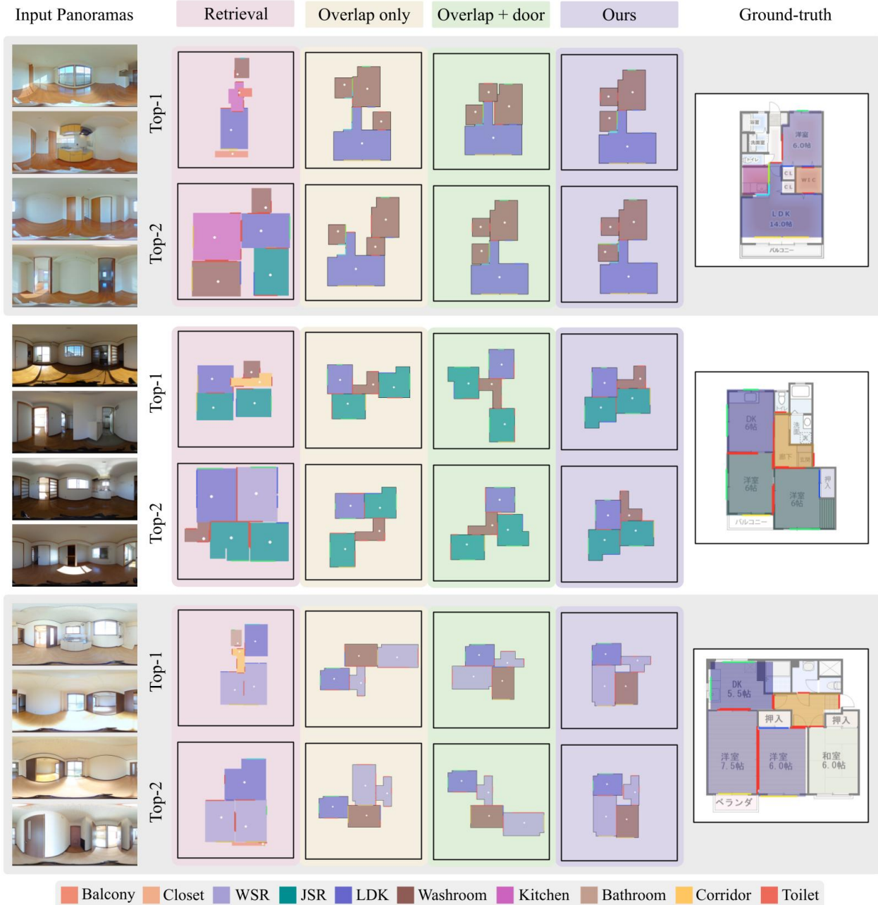
Figure 8. Qualitative comparisons against the three competing methods. We show the top-2 reconstructions from each method based on their scoring functions. Room colors indicate their types
