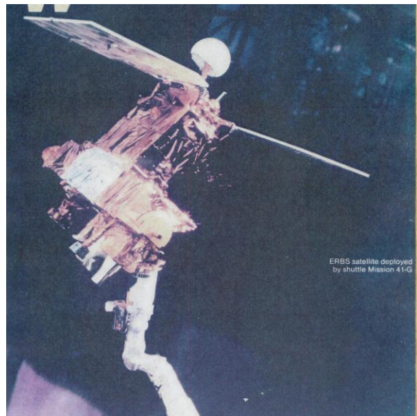
Figure 3: ERBS held by Remote Manipulator Arm of Challenger before release into space.
