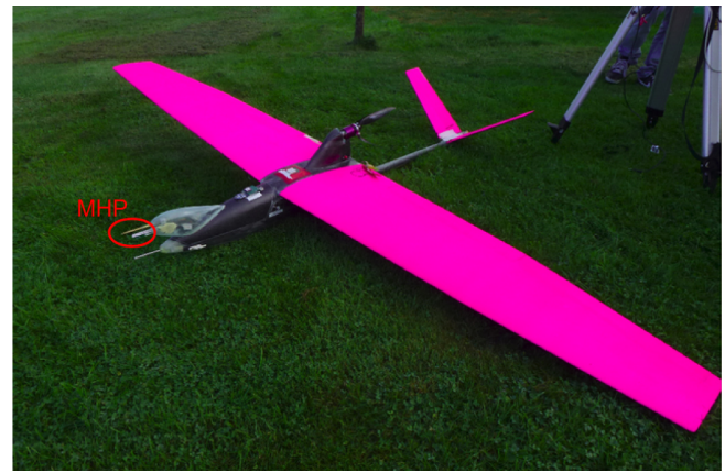
Fig. 1. Research RPA MASC. The position of the MHP approximately 15 cm in front of the fuselage nose tip is depicted with the red ellipse.
