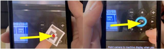
Figure 4: TutorialLens records the 3D coordinates of the finger locations relative to the device marker in the authoring mode, and reproduces the finger location corresponding to the current device marker in the access mode.
