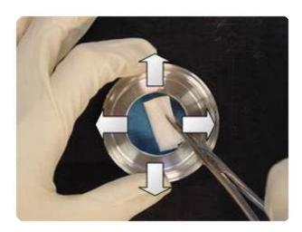
Note:- Extreme care should be exercised to ensure that the forceps do not make contact with the window.
