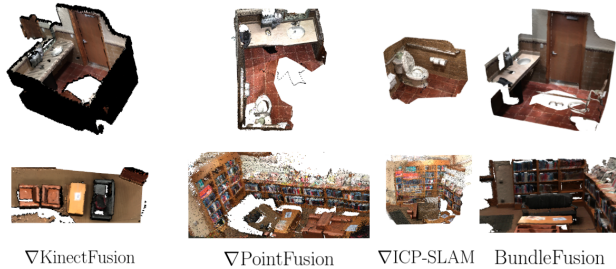
Figure 2. Qualitative results on sequences from the ScanNet [4] dataset. We use each of the differentiable SLAM systems ( \nabla KinectFusion, \nabla PointFusion, and \nabla ICP-SLAM) to reconstruct parts of the scene. We also show outputs from BundleFusion [5].
