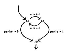
From this it can be deduced that the L1-L3 loop does not alter *parity*, and that after this loop exits to L2 control cannot pass back to the loop, and so that PARITY need not be an argument to L1 or L3 in the SCHEME version.
