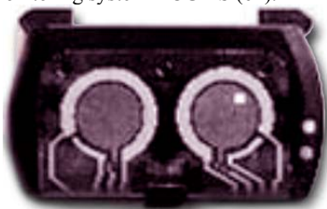
Figure 10. The extracted glucose is measured by an amperometric biosensor (AutoSensor) using detection of H_2O_2 generated by the glucose/glucose oxidase reaction (63-65).
