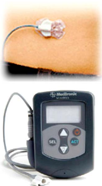
Figure 9. (Upper): Medtronic/MiniMed continuous Subcutaneous Glucose Sensor and (bottom): a continuous glucose monitoring system – CGMS (61).
