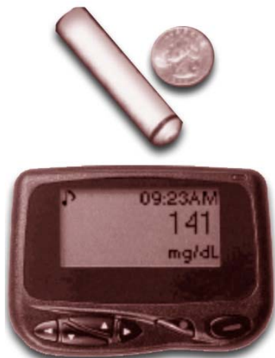
Figure 11. Upper: Implantable glucose sensor the size of a AA battery. Bottom: The receiver is an externally worn pager-sized device. Sensor glucose data are transmitted wirelessly from the sensor to the receiver (66).
