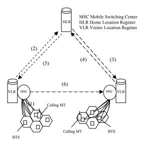
Figure 5: Call delivery procedure
