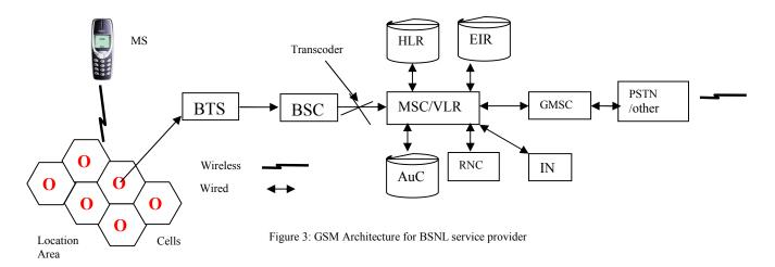
*Base Station* (BS): The base station is the gateway between the wireless network and wired network. It provides the wireless connection to the mobile subscribers within its coverage area (Cell). A set of base stations are connected to the MSC through a Base Station controller.
