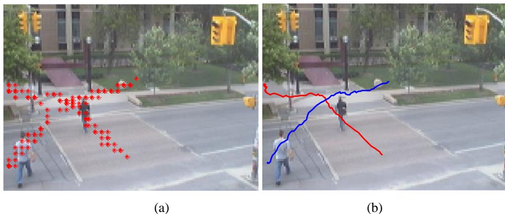
Fig. 5. Detection and tracking of multiple moving objects: (a) detected objects (represented in red dots); (b) tracking of two detected objects with occlusion.
