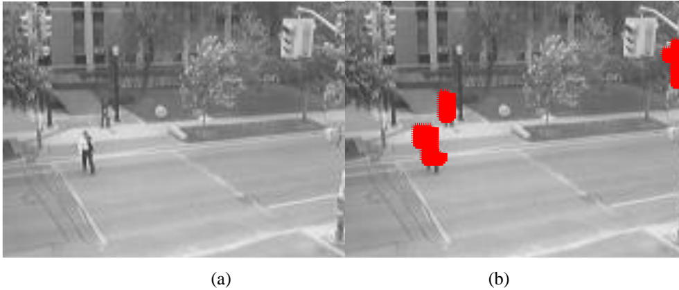
Fig. 4. Moving object detection: (a) an exemplary image of original input image sequence; (b) detected moving objects.
