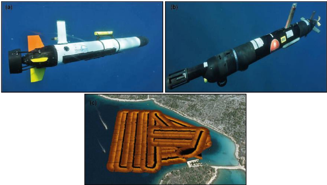
Fig. 10. (a) Klein-3500 side-scan sonar attached to AUV IVER2, (b) Yellow-fin side-scan sonar attached to AUV LAUV, and (c) The study area and the AUV path (Vasilijevic et al.) [104].
