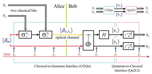
**Figure 6.** SDC protocol and the detail of its constituent interfaces.
