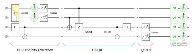
**Figure 10(a).** SDC  $\equiv$  Cl2Qu  $\cup$  Qu2Cl on Quirk® for  $\{b_1,b_2\}=\{0,0\}$ .
