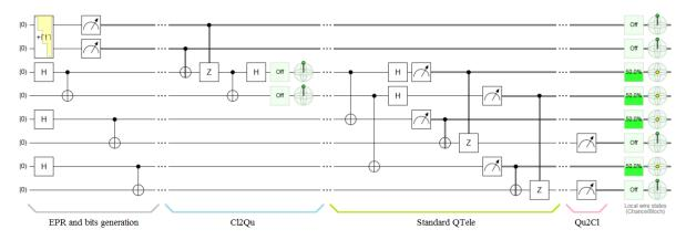
**Figure 13(a)**. Standard QTele on Quirk® of a pair  $\{b_1,b_2\}=\{0,0\}$ .
