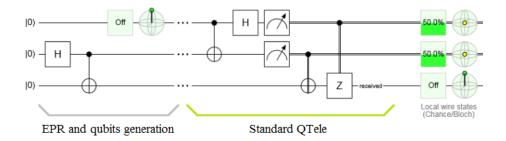
**Figure 11(b)**. Standard QTele for the teleportation of  $|0\rangle$ .
