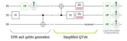
**Figure 12(b)**. Simplified QTele for the teleportation of  $|0\rangle$ .
