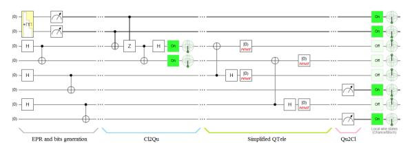
**Figure 14(d)**. Simplified QTele on Quirk® of a pair  $\{b_1,b_2\}=\{1,1\}$ .
