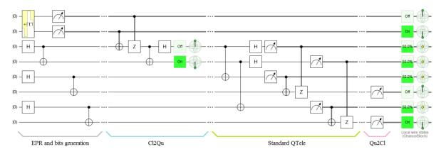
**Figure 13(c)**. Standard QTele on Quirk® of a pair  $\{b_1,b_2\}=\{1,0\}$ .
