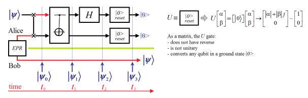
Figure 5. Simplified teleportation protocol using an EPR pair but without classical bits for disambiguation.
