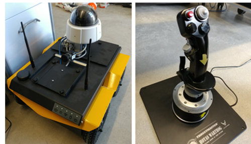
Fig. 11 Jackal UGV robot from Clearpath Robotics Inc. (left) and a gaming joystick (right).
