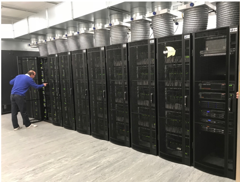
Figure 1. The million-core SpiNNaker machine at the University of Manchester, occupying 10 rack cabinets with an 11 th cabinet (shown on the right) containing the associated servers.
