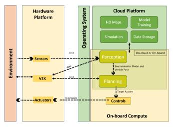
FIGURE 5 Orchestration of Hardware, Software, Cloud and Onboard compute platforms where Autonomy Block technology operates.
