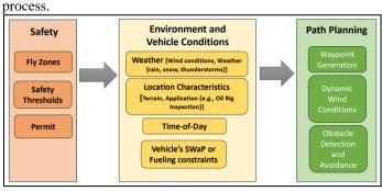
FIGURE 4 Three stage process of Mission Planning
