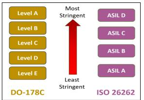
FIGURE 12 DO-178C and ISO 26262 comparison.
