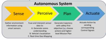
FIGURE 2 Four Major Building Blocks of Autonomous Systems
