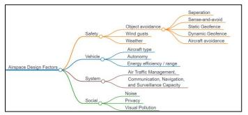
FIGURE 10 Factors influencing the design of UTM operations.
