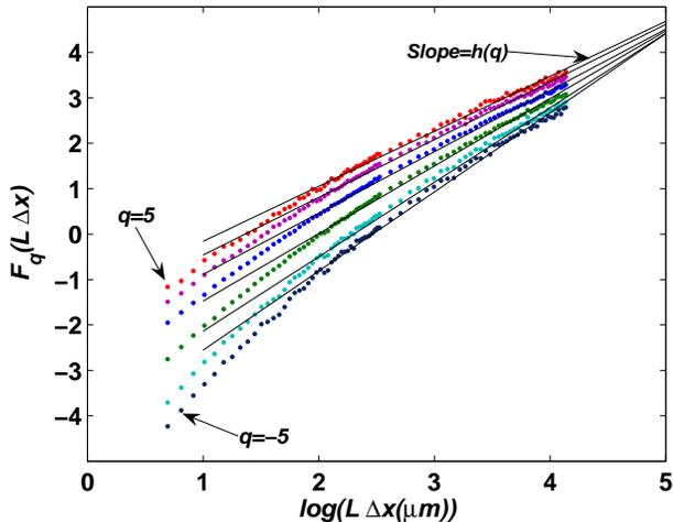
FIG. 3: The logarithm of the fluctuation function  $F_q(L\Delta x)$  as a function of the logarithm of the distance  $d = L\Delta x$ , for Py29 sample, for  $q = -5, -3, -1, 1, 3$  and  $5$ . The straight lines are the regression fits to the data at large scale. The slopes of the lines determine  $h(q)$ .
