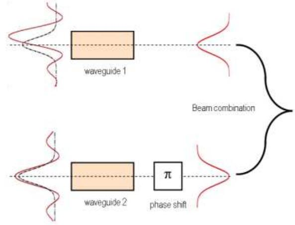
**Fig. 1.** Schematic view of modal filtering of the interferometric beams *before* recombination. By tilting the wavefront in one channel, the coupling efficiency is degraded. This impacts only the amplitude of the fundamental mode, not its phase.
