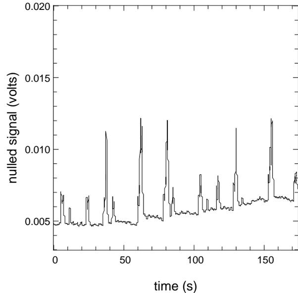
**Fig. 5.** Nulled output as a function of the time. This plot shows that the time scale over which the null can be considered stable is 10 to 20 seconds. The strong spikes come from sensitivity of the setup to vibrations and external constraints.
