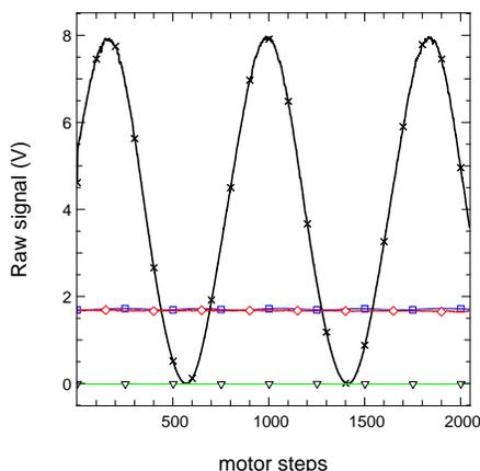
**Fig. 3.** Raw signals as a function of motor steps involved in the dynamic measurement of the interferometric null. The black curve (crosses) is the interferometric signal. The blue (squares) and magenta (diamonds) curves are the photometric channels. The green curve (triangles) is the detector offset. One scan has 2048 points recorded over 190 s. The linear step is 12 nm.
