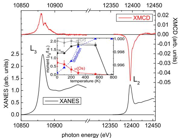
Figure 3: (Color online) XANES (left axis) and XMCD signal (right axis) at the Os  $L_2$  and  $L_3$  edges in  $\text{Sr}_2\text{CrOsO}_6$ . The inset shows the element resolved magnetic moments of Cr ( $\mu_{\text{Cr}}$ ), Os ( $\mu_{\text{Os}}$ ), the total magnetic moment ( $\mu_{\text{tot}}$ ) and the lattice distortion as determined from neutron scattering data refinement (see Table II).
