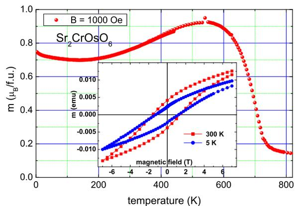
Figure 2: (Color online) Magnetization vs temperature and hysteresis (at 5 K and 300 K) of  $\text{Sr}_2\text{CrOsO}_6$  (measured in a superconducting quantum interference device (SQUID)). The sample has been cooled and field-oriented in diamagnetic  $\text{LiNO}_3$  (melting point 480 K) because of the high anisotropy field.
