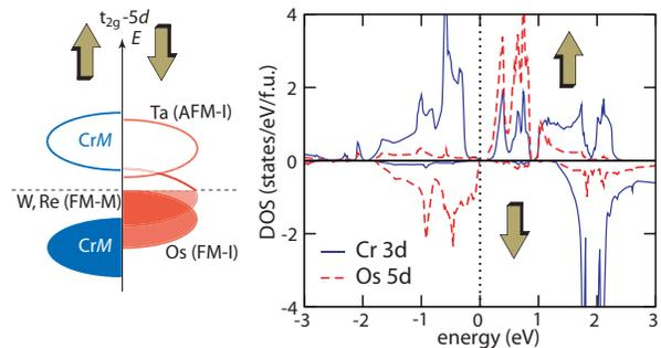
Figure 4: (Color online) Left: Band structure sketch for different fillings of the  $5d$  spin-down band (as realized in the materials  $\text{Sr}_2\text{CrMO}_6$  with  $M = \text{Ta}, \text{W}, \text{Re}, \text{Os}$ ). Right: Band-structure calculation for  $\text{Sr}_2\text{CrOsO}_6$  using the generalized gradient approximation including spin-orbit coupling (GGA+SO).
