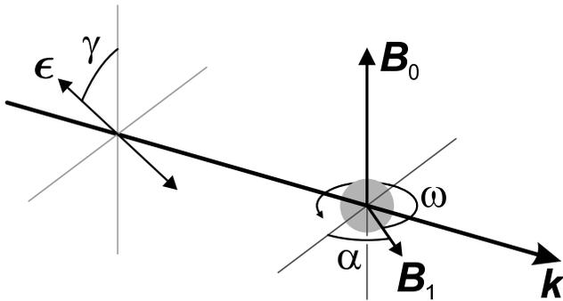
FIG. 1: Double resonance magnetometer geometry using linearly polarized light. Here,  $\mathbf{k}$  is the direction of the linearly polarized laser beam. The rf field  $\mathbf{B}_1$  (shown here at  $t = 0$ ) rotates in a plane perpendicular to the static field  $\mathbf{B}_0$ . The linear polarization vector  $\epsilon$  makes an angle  $\gamma$  with the static field  $\mathbf{B}_0$ , and the phase of  $\mathbf{B}_1$  is characterized by  $\alpha$ .
