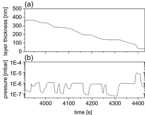
Fig. 10. Controlled sublimation of SXe layers. Panel (a) shows the layer thickness as a function of time. The pressure in the vacuum chamber during controlled sublimation is shown in panel (b).
