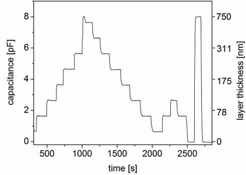
Fig. 8. Dynamically stabilized solid Xe layers grown and sublimated at constant pressure of 700 mbar Xe gas, using a sensor type 9 and active feedback on the capacitance of the sensor. The left and right scales are, respectively, the sensor capacitance and thickness. At 7.98 pF the sensor response saturates. Stable layers are, again, obtained for periods of many minutes.
