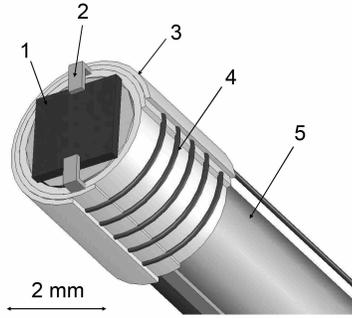
Fig. 2. Diced 2 mm diameter sensor (1) mounted at the end of the copper cold finger (5) of the miniaturized cryostat. The readout pads of the sensor are contacted by gold coated leads (2). An assembly of three Vespel sleeves (3) holds the leads and the tungsten heater wire (4) in place.
