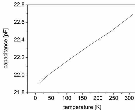
Fig. 4. Capacitance of a sensor during cooling from room temperature to about 15 K in  $2 \cdot 10^{-8}$  mbar (300 K) vacuum. The capacitance is the sum of the unshielded sections of the readout cables (0.7 pF) with the dielectric constant of vacuum. The fluctuations of the measurement are smaller than the line width in the plot.
