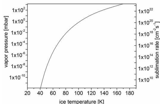
Fig. 6. Calculated vapor pressure of solid Xe at different temperatures. On the right scale the expected sublimation rate of Xe atoms based on the Hertz-Knudsen model in vacuum is shown.
