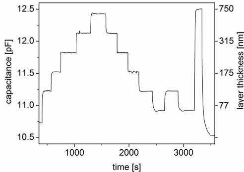
Fig. 9. Solid frozen from LXe, using a sensor type 10 and active feedback. At 12.5 pF the sensor saturates. The offset of 10.52 pF is due to the dielectric constant of LXe.
