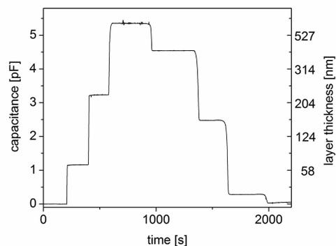
Fig. 7. Capacitance of a type 5 sensor with different thicknesses of solid Xe in  $< 3 \cdot 10^{-8}$  mbar vacuum. The solid Xe is deposited on the sensor, which is kept at  $< 30$  K, by condensing a known amounts of gas. Sublimation is obtained by increasing the temperature of the sensor. The plateaus correspond to stable frozen Xe layers.
