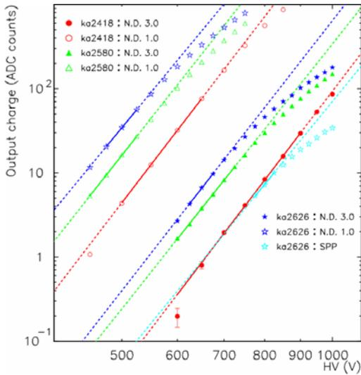
Figure 8.8: Measurements of PMT output versus applied high voltage.
