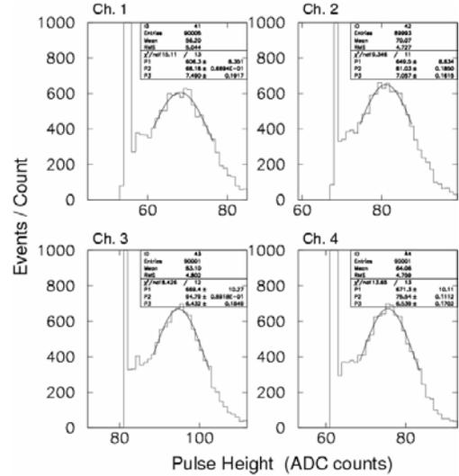
Figure 8.9: Pulse height distributions with very low light level (approximately 0.1 photoelectrons)
