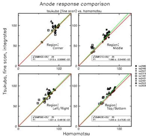
Figure 8.7: Comparison of the integrated anode responses from the Tsukuba fine-scan to the Hamamatsu anode uniformity data.
