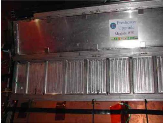
Figure 1.2: Picture of the front face of the inner calorimeter arch, showing three wedges. The middle wedge is bare, showing the front of the electromagnetic calorimeter. The bottom wedge has the old gas preshower detector which was replaced; the top wedge has the new preshower detector.
