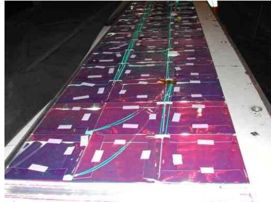
Figure 1.3: Picture of a CPR module before the top cover was installed, showing the individually wrapped tiles and fibers exiting them.
