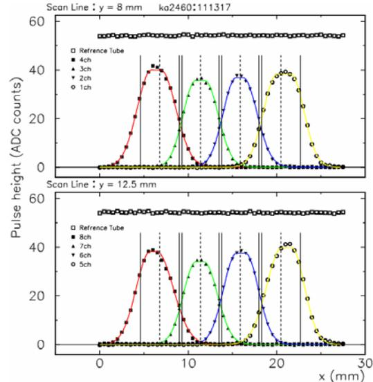
Figure 8.6: Response of four channels in a given row of a PMT as a function of the illumination position  $x$  while keeping the position  $y$  near the center of the pixels.
