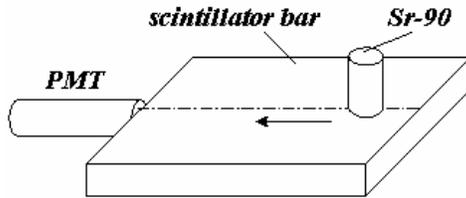
Figure 4.2: Schematic view of the source measurement setup.
