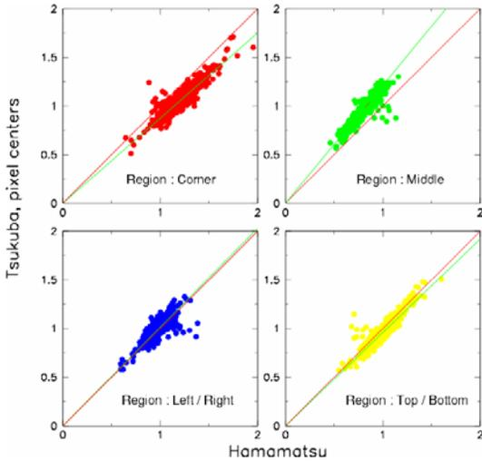
Figure 8.4: Comparison between Tsukuba measurements of responses at the center of 16 channels with that from Hamamatsu anode uniformity data, for 200 PMTs. The four subplots correspond to the four regions of the PMT.
