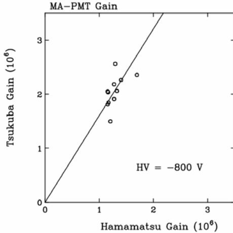
Figure 8.10: Comparison of PMT absolute gains measured at Tsukuba with those from Hamamatsu data sheet values.
