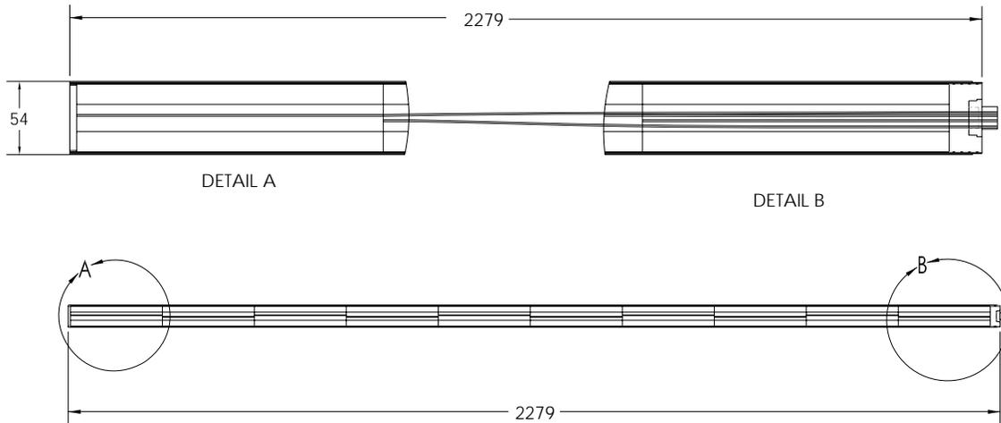
Figure 3.3: Top view of the CCR module, with only 2 fibers shown for clarity.
