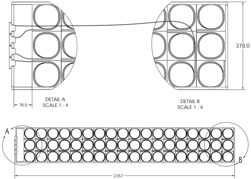
Figure 3.2: Top view of the CPR module, with only 1 fiber shown per connector for clarity.
