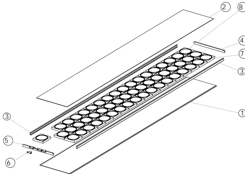
Figure 3.1: The CPR module with the fibers not shown. 1-2) Top/bottom aluminum covers, 3) aluminum U-channels, 4) PVC back piece, 5) PVC connector holder, 6) example connector for fibers, 7) scintillator tile, 8) groove for fibers.
