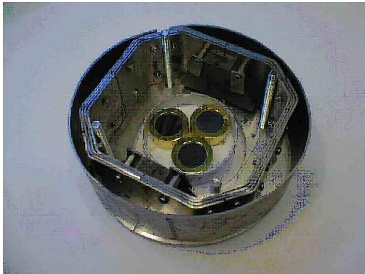
**Fig. 16:** Three  $300 \text{ mm}^2$  ULTRA detectors used for spin polarisation analysis are set within an array of permanent magnets
