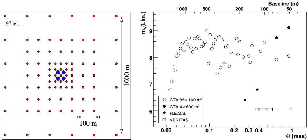
**FIGURE 1.** *Left:* Proposed lay-out for the future CTA. The small dots are the 85  $100\text{m}^2$  dishes, the large dots are the 4  $600\text{m}^2$  dishes. *Right:* I.I. with CTA sensitivity estimate as function of the 47 non-redundant baselines for a  $5\sigma$  detection, in a 5 hours integration on a star with 50% visibility. Final values depend on signal bandwidth and CTA design details (see Le Bohec et al., these proceedings).
