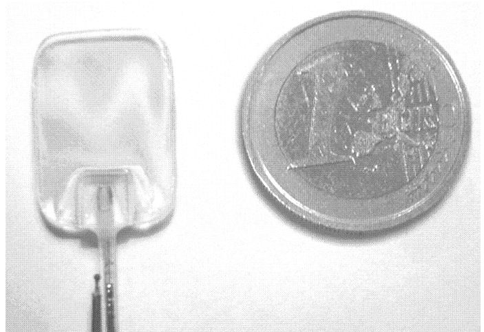
FIG. 8: Photograph of a nanocell filled with Na. A 1 Euro coin is shown for the scaling.
