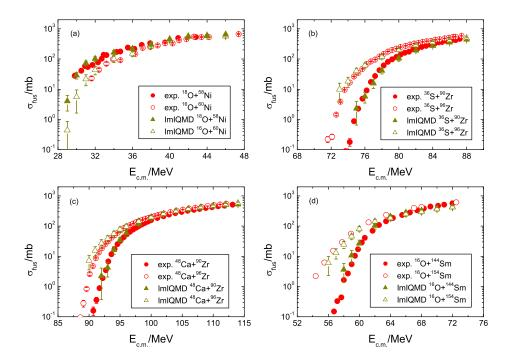
Figure 9: Comparisons of the calculated fusion excitation functions and experimental data for a series of reaction systems.
