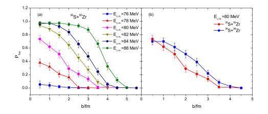
Figure 6: The fusion probability as a function of the impact parameter and its dependence on the incident energies and on the system size.
